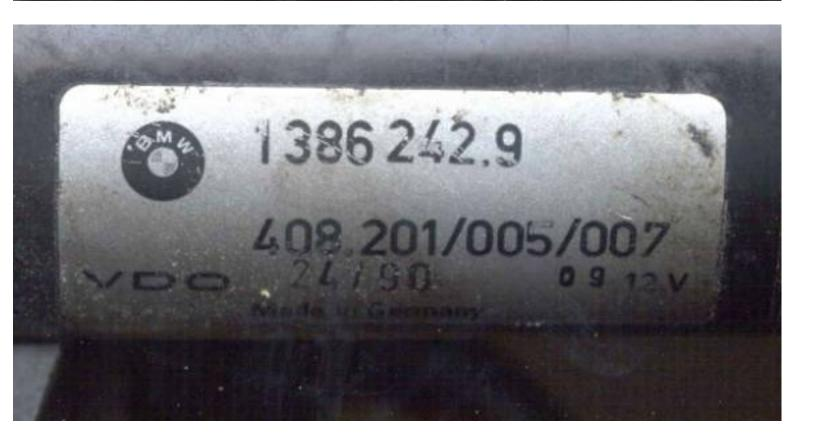
Black plastic box with a motor mounted on it. Has two cables coming out of it, one with a grommet and a 7 pin electrical connection on the end, the other with a linkage identical to the one that is used for the gas pedal cable/throttle arm.
