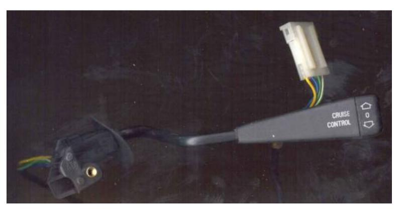
Turns the cruise on and off, sets and resumes speed. Looks like the windshield washer lever, but has cruise commands on it.
