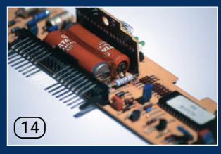
9 And here's one we removed earlier, which explains the different coloured batteries. You'll see that not only are the batteries soldered to the circuit board but they're glued in place too. Luckily this glue is normally brittle with age and doesn't make it difficult to remove them.
