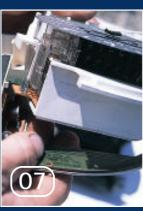
First step is to remove the instrument cluster from the car. Your workshop manual will tell you exactly how to do this, but on the E28 it's simple. Just use a fine crosshead screwdriver to remove the two screws under the top edge of the instrument cowling and then a large screwdriver to prise the top edge downwards until the unit pops out. Wiggle it forwards and the electrical connectors will be exposed.
