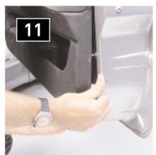
6 Twist and pull the door locking button until it comes free. It doesn't look important but you can't get the door trim off without removing it.
