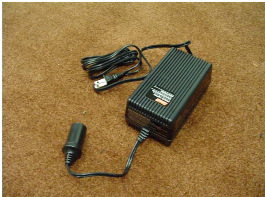
Start with one wire, hooking one side of the power supply to one wire and the other side of the power supply to one your test instrument. Then touch the other side of your test instrument to each wire until you get a reading. Do this also while holding in one button at a time. I.E. – Hold in the white arrow and see what wire lights up. Keep trying different wires until you can fill this chart:
