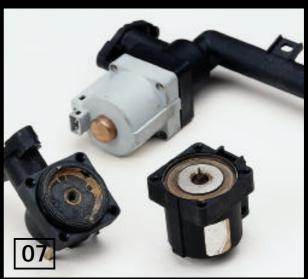
New valves are available for about £40 from suppliers like German & Swedish and Euro Car Parts. When fitting a new one, grease the 0-ring where the valve fits on to the matrix and don't forget to make sure the grommet where the valve pokes out into the engine bay is intact.
