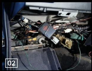
Now drop the glovebox down and disconnect the two straps after removing the top plastic cover above the glovebox. Do this by twisting the top plastic lugs through 90 degrees, pushing them up and then out. It's tricky. With the glovebox dropped right down, remove the plastic cover to the side of the glovebox, followed by the plastic trunking. This can be a real pain to get out, but once removed you can see the heater valve easily.
