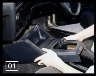
Whatever the fault, the first thing to do is remove the valve and test it. Firstly, remove the centre console. There's a plastic nut at the rear behind the handbrake lever under a cover and with that removed, the rear console pulls backwards and off. The main console is held on with another plastic nut under the gearlever gaiter and two 8 mm bolts going up into the main facia. Remove the console after disconnecting the wires for the cigarette lighter.
